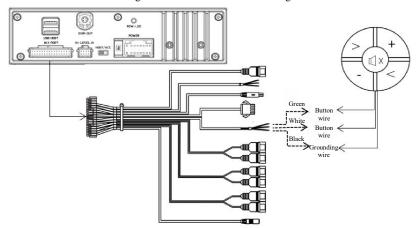
\*Connect the green and white wires with the button wires of the steering wheel and connect the black wire with the grounding wire. Please connect the wires based on the actual vehicle model. For details, please
