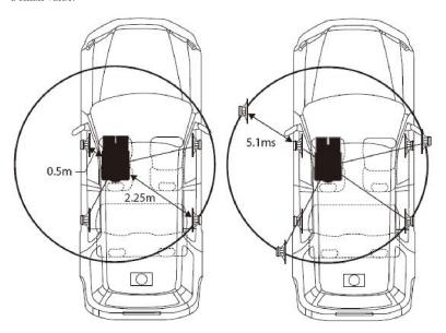
The distances between the listener location and the speakers are different, and therefore the sound is not balanced.
