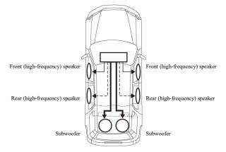
Frequency range is output with high/medium frequency for the front speaker and low frequency for the bass speaker.
